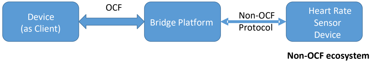
414 415 Figure 1 – Server bridging to Non- OCF device
