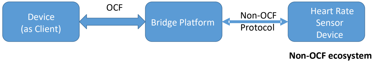
329 330 Figure 1 – Server bridging to Non- OCF device
