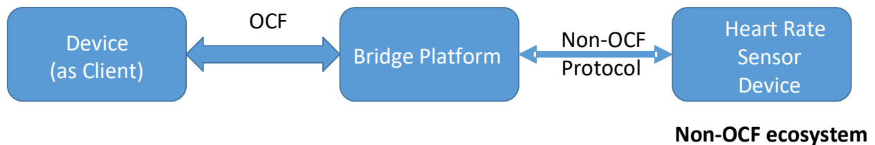
Figure 1 – Server bridging to Non- OCF device
