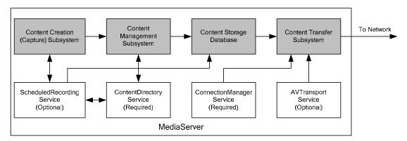
Figure 1: MediaServer Functional Diagram
