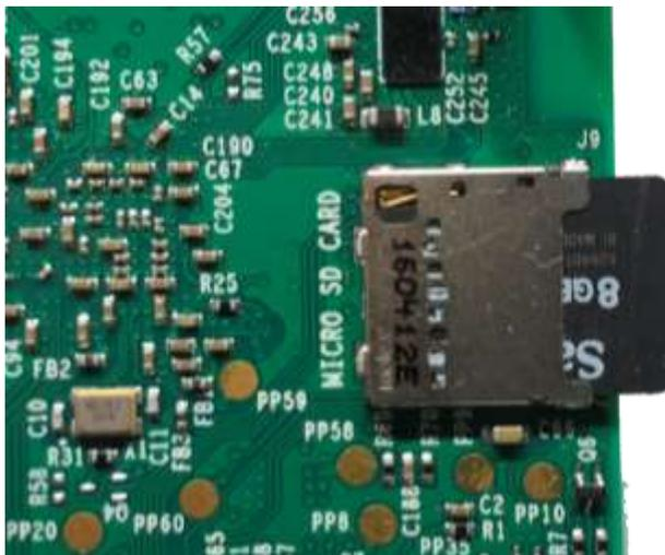
The microSD card in the kit has been formatted and loaded with a bootable Raspbian Stretch Lite OS, configured with SSH enabled. This version of Raspbian does not include
