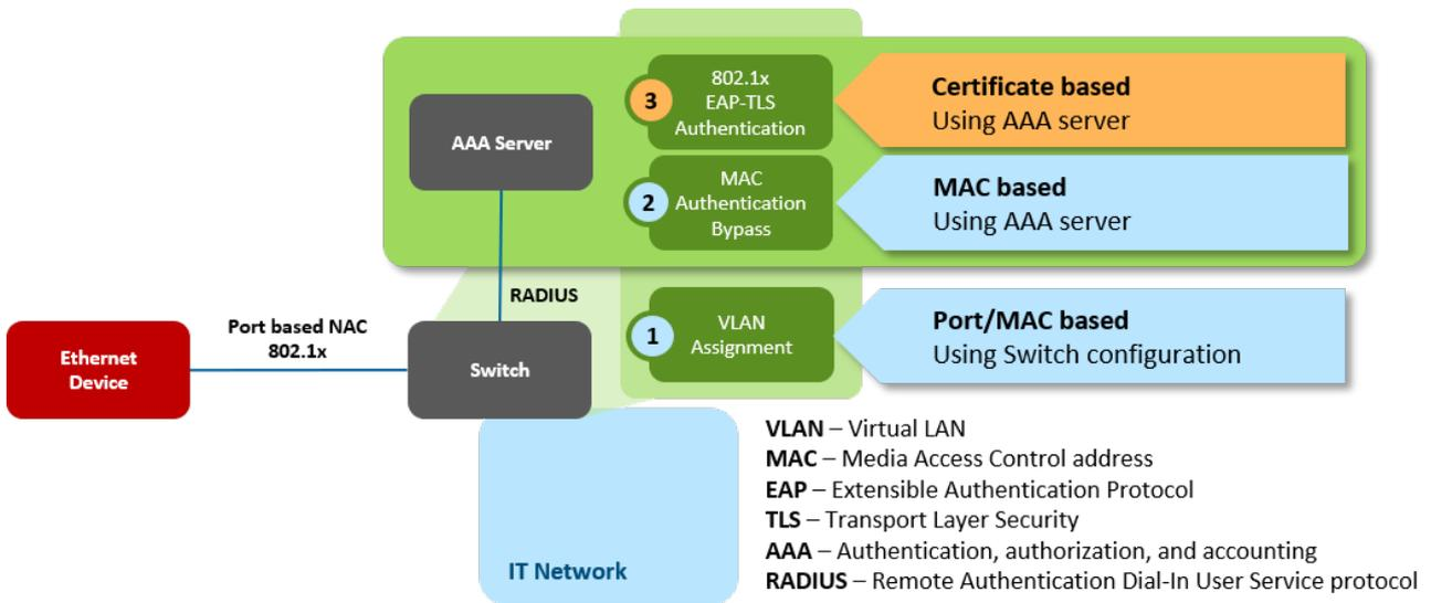
Figure 8: Network Access Control options for Ethernet devices
