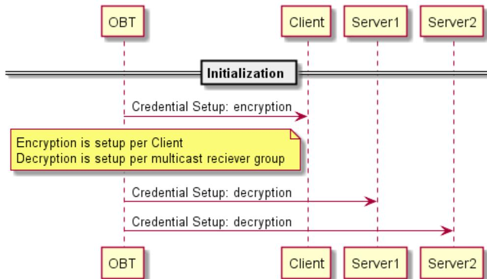
**Figure 2 Configuring Secure Simple Multicast**
