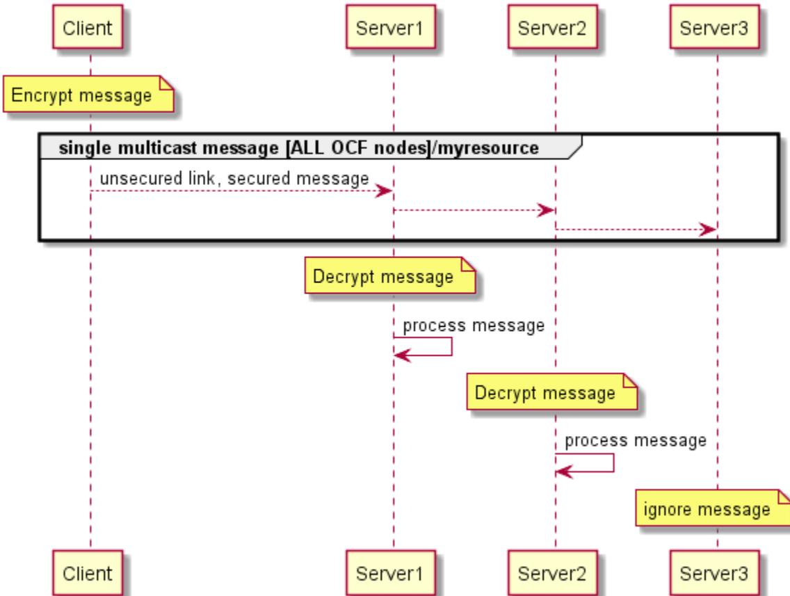
**Figure 1 Sending Secure Simple Multicast messages**
