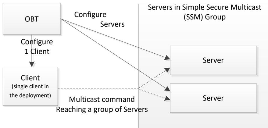
**Figure 1 Schematic overview of SSM group communication**
